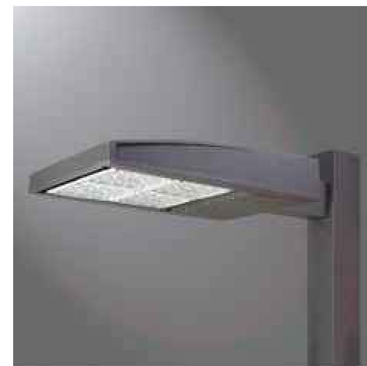
Parking Lot Light MFR: McGraw-Edison Model: Galleon LED area and roadway luminaire 70 CRI, 4000K, 1A Lightsquares and spill light eliminator optics with house side shield
